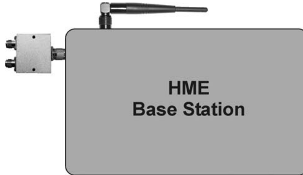
Figure 3. Splitter on base station antenna connector
